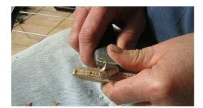
11. **Cut the tail section in**, being very careful not to cut yourself – a leather nail bag provides good protection. Start the cut about a  $\frac{1}{3}$ rd of the lure length from the tail.
